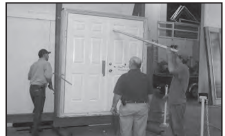
DP Structural Testing
